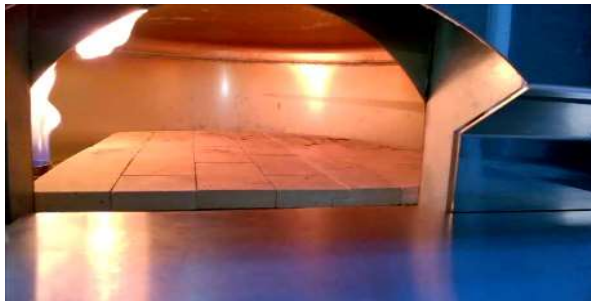
Fixed Cooking Refractory Floor
