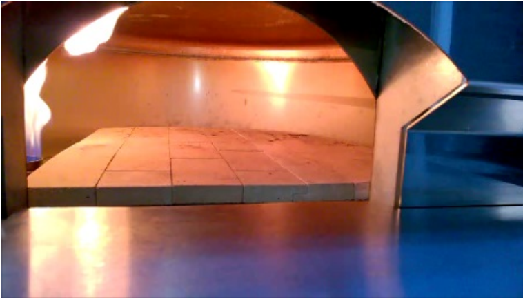
Fixed Cooking Refractory Floor
